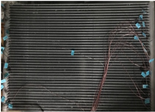
图 2 微通道蒸发器实物和温度测点示意图 Fig.2 Schematic diagram of MCE and temperature test point
